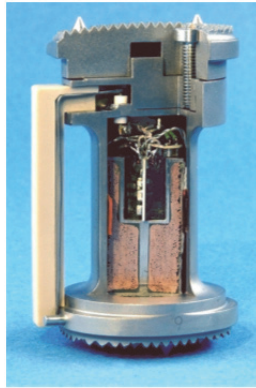
Fig. 25. Wireless load measuring system for vertebral body replacement (Rohlmann et al., 2007)
